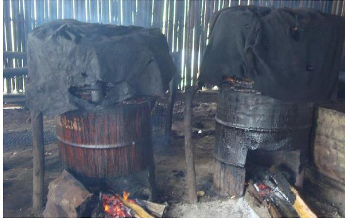
**Plate8.** *Traditional Cut-Drum Fish Smoking Oven*
