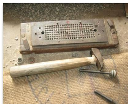
Plate2. Hammer for cutting the punch card
