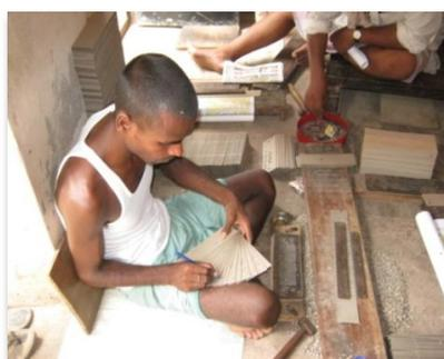
Plate3. Punch card cutter giving sequential number
